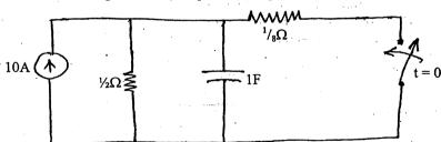
b) In the network shown, the switch is closed at t = 0. Find the current supplied by the source using Laplace transform method.
