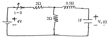
3. a) In the circuit shown switch is opened for a long time and then it is suddenly closed at t = 0. Obtain the expression for current through inductor for t > 0. Also calculate the voltage across inductor after 10mSec. [Use classical method]
