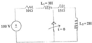
b) Calculate expression for total current supplied by source for t > 0 using classical method in the circuit shown below.
