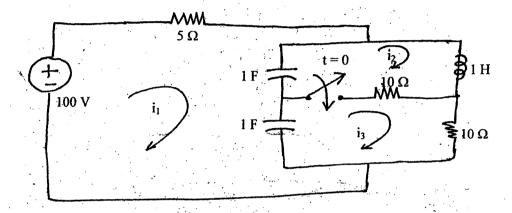
2. a) Find  $v_a(t)$  for t > 0 in the figure below using classical method.
