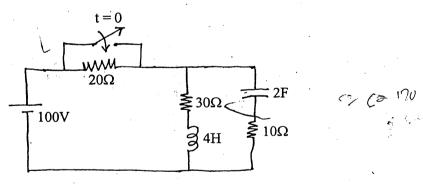
b) At t = 0, switch is closed in the circuit of figure below. Find the  $V_c(t)$  and  $i_c(t)$  using classical method.
