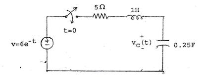
3. a) In the network shown, the switch is moved from 1 to 2 at t=0. For the element value given on diagram, find the expression for voltage and current of capacitor, by Laplace Transformation method.
