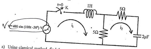
2. a) Using classical method, find the expression for the current supplied by the source in the network shown in figure. Also find the time taken by the source current to reach
