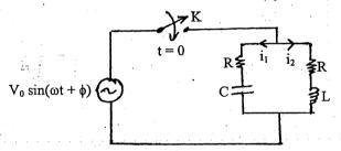
2. a) In the given circuit, after the switch has been in the open position for a long time, it is closed at t = 0. Find the voltage across the capacitor using classical method.
