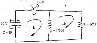
4. a) For the 2-port network shown in figure below, find voltage ratio transfer function, G<sub>21</sub>(S) and transfer admittance, Z<sub>21</sub>(S). [8]
