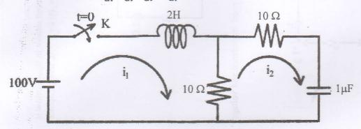
a) In the circuit shown in figure below, if the switch is closed at t = 0, find the expression for voltage across capacitor using classical method. [8]
