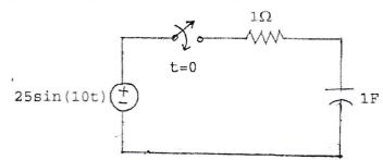
b) Obtain an expressions for V<sub>c</sub>(t), if the switch in the circuit shown in figure below is closed at t=0. Use Classical method.
