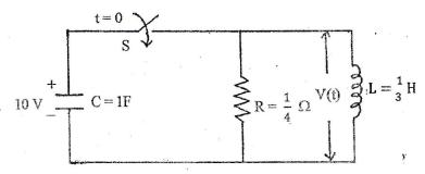
3. a) Using Laplace transform method find the current through the inductor in the network shown in figure below.
