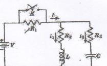
a) Find the forward voltage ratio transfer function G<sub>21</sub>(s) and forward transfer admittance Y<sub>21</sub>(s) in the following circuit.
