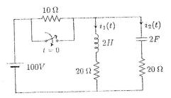
2. a) In the two mesh network, the switch is closed at t=0. Find the mesh currents i<sub>1</sub>(t) and i<sub>2</sub>(t) using classical method. Also calculate the capacitor voltage. [8]
