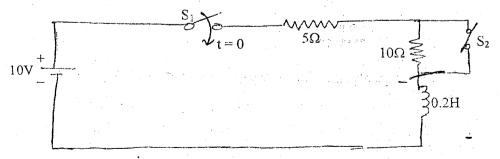
b) The circuit shown below is in steady state with switch 'S' closed. The switch is opened at t = 0. Using Laplace Transform method, find  $i_L(t)$  in the circuit. [8]
