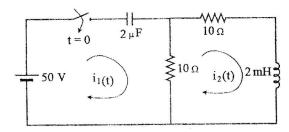
2. a) Using classical method, find current and voltage across capacitor for t > 0 in the circuit shown below.
