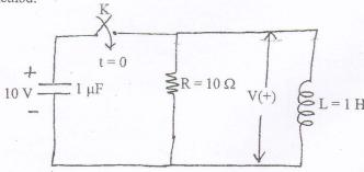
3. a) Using Laplace transform method find the expressions for  $i_1(t)$  and  $i_2(t)$  in the given two mesh network shown in figure below provided that the network is unenergised.
