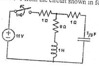
3. a) In the series R-L-C circuit shown in figure, there is no initial charge on the capacitor. If the switch S is closed at t=0, determine expression of current and voltage for all elements for t>0.
