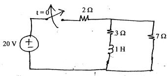
b) Using Laplace transform method, find he loop currents i<sub>1</sub> and i<sub>2</sub> for t > 0 in the circuit shown in the following figure. [8]
