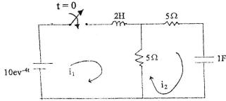
2. a) Using classical method, find the voltage across inductor L<sub>2</sub> in the circuit shown in following figure.
