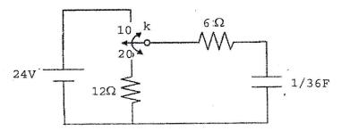
b) In the circuit shown in figure below, if the switch is opened at t=0, find  $V_c(t)$  for t>0, using Laplace transform method.
