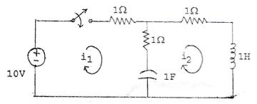
2. a) If the switch is closed at t=0 in the circuit shown in figure below, find expressions for current through and voltage across capacitor using classical method of solution.
