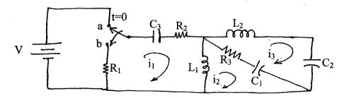
b) Switch in the circuit is suddenly opened at t = 0 after steady state has been reached in the closed position of the switch. Use classical method to determine the expression for voltage across capacitor for t > 0.
