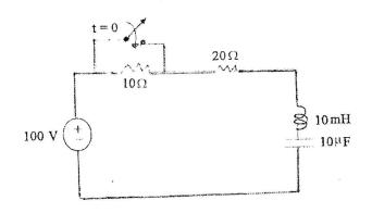
3. a) Using Laplace Transform method, find the current and voltage across capacitor for t > 0 in the circuit shown below.
