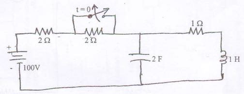
3. a) Using Laplace Transform method in the circuit shown in figure below find the voltage and current of capacitor for t>0
